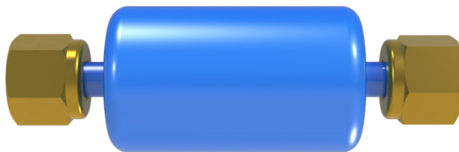
FIGURE 9-1. The vortex filter assembly includes a 25 µm particulate filter with 1/4-in Swagelok nuts on either side.
